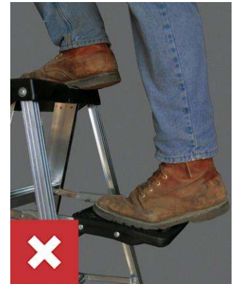
WRONG DON'T climb on the back of a stepladder. DON'T stand or sit on a stepladder top or rail shelf.
