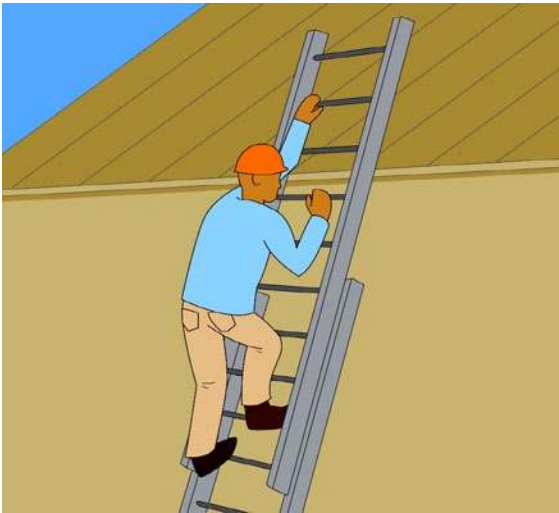
Figure 2: Ladder extending three feet above the landing area.
